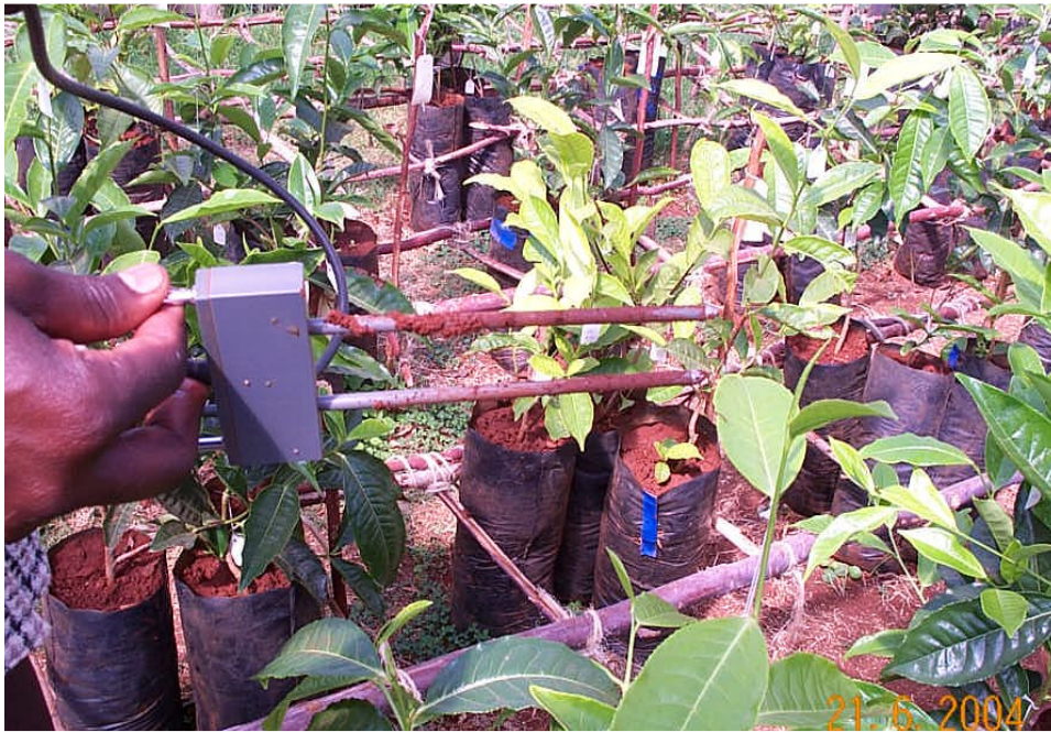
Plate 4.2 Trime FM2 probe used for soil water content determination in the experiment.
