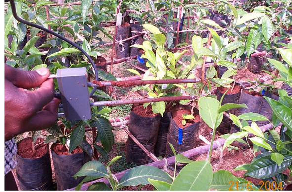
Plate 3.3 (b) Soil moisture meter probe used in the study.
