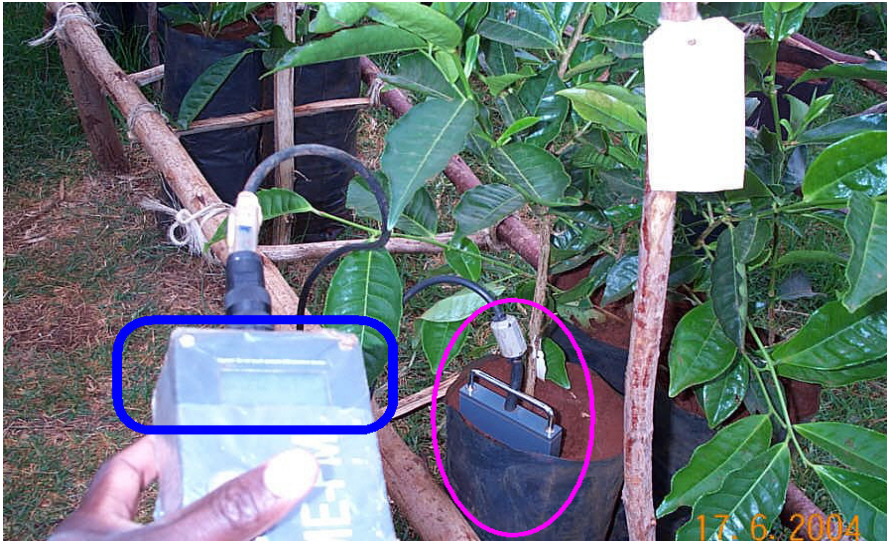
Plate 4.1 Trime FM2, TDR soil moisture meter inserted in soil and soil water content indicated on read-out circled with blue.
