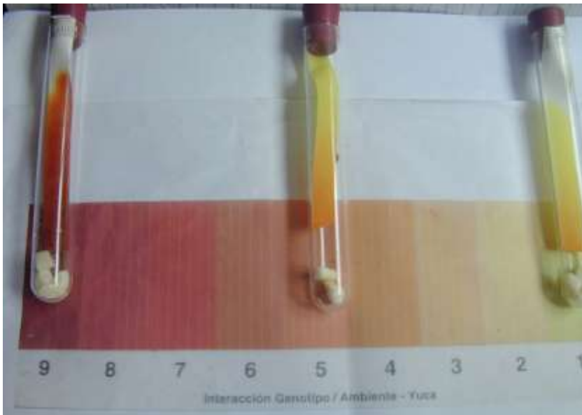
Figure 2: Color chart for cyanide analysis of cassava accessions using modified picrate testing procedure.
