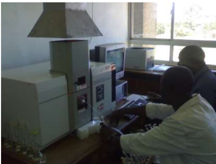
Figure 3: Analysis of cassava accessions using Atomic Absorption Spectrophotometer (Shimadzu Model AA-6300, Tokyo-Japan).
