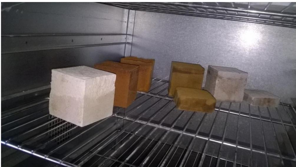
Plate A.10: Oven Dry samples at 1100C
