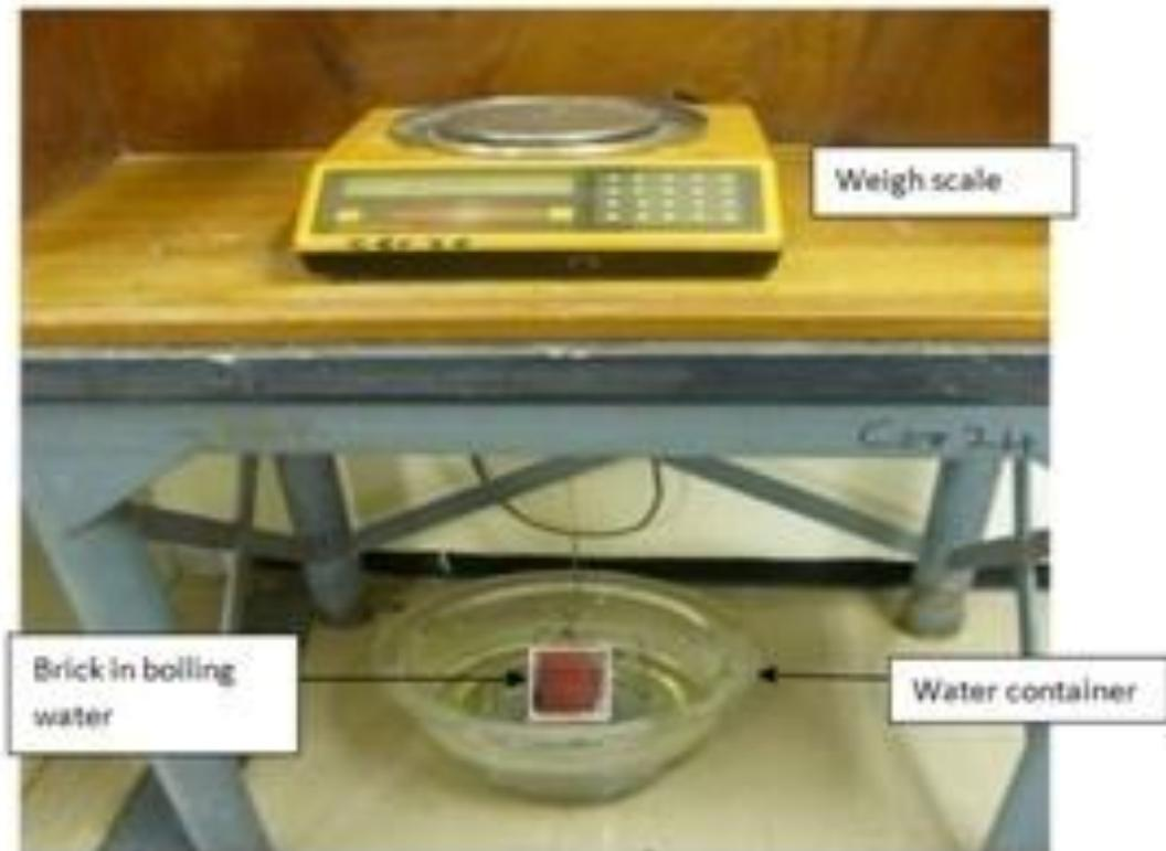
Plate A.12: Apparent porosity and bulk density testing equipment
