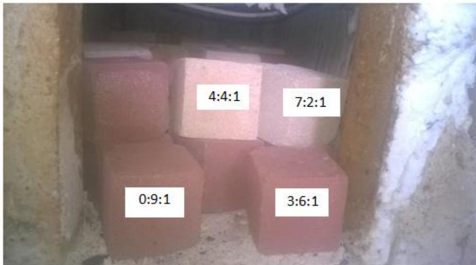
Figure 4.4: Fired bricks samples at different mix ratios.
