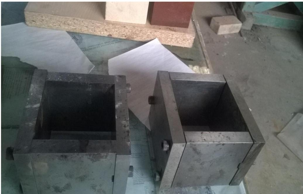
Plate A.8: Cubical mould box of side 70 mm.
