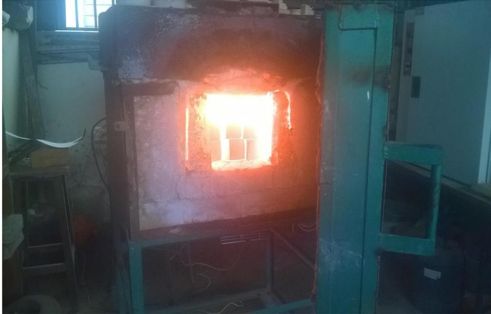
Plate A.11: Samples in automatic digital electric furnace
