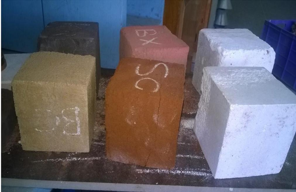
Figure 4.2: Fired bricks of individual clays.
