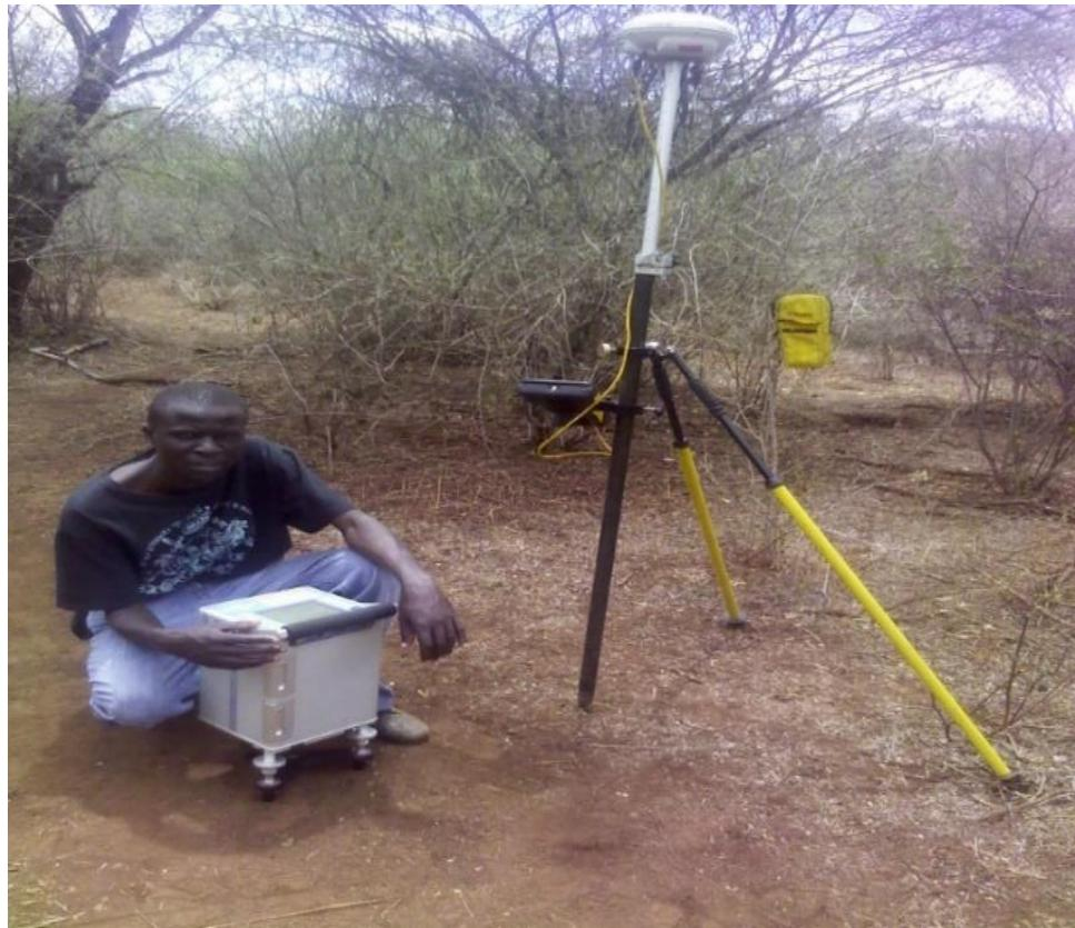
**Figure 3.3:** Gravity measurement being taken in the field using a gravimeter and DGPS receiver.
