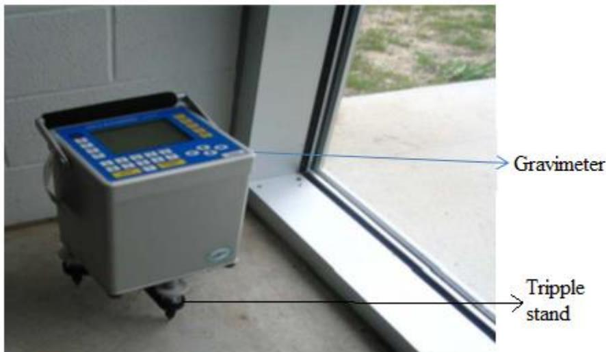
**Figure 2.1:** CG-5 Autograv gravimeter
