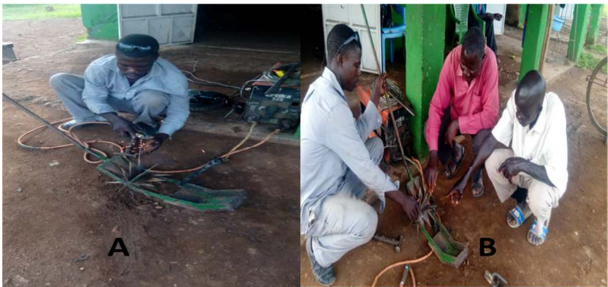
Plate 10: Local ‘Jua-Kali’ Artisan fabricating push-weeder (A). Artisan receiving advise from experienced SRI farmers how to modify the push-weeder blades (B)
