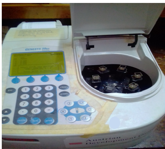
Plate 3: A photo of spectrometer used for reading absorbance which help to determine concentrations
