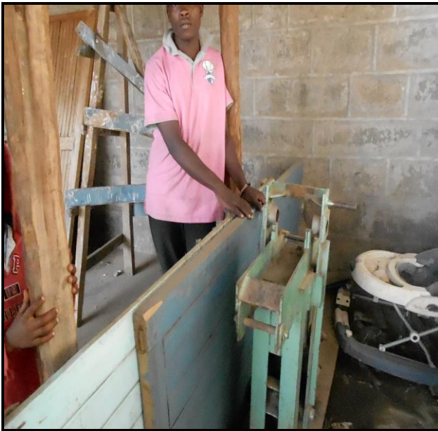
Plate 4.5.13: Broken-Down SSB Machine in Kwa Rhonda Project Site
