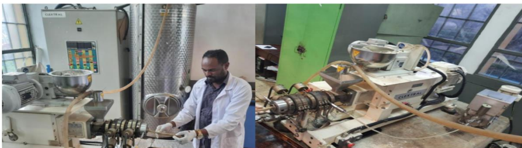
Figure 5.1. The extrusion machine used for this study
