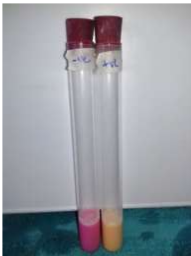
Figure 7: Colour observations using ingredients as powder on a Beta-lactams positive (right test tube) and a negative (left test tube) raw milk sample
