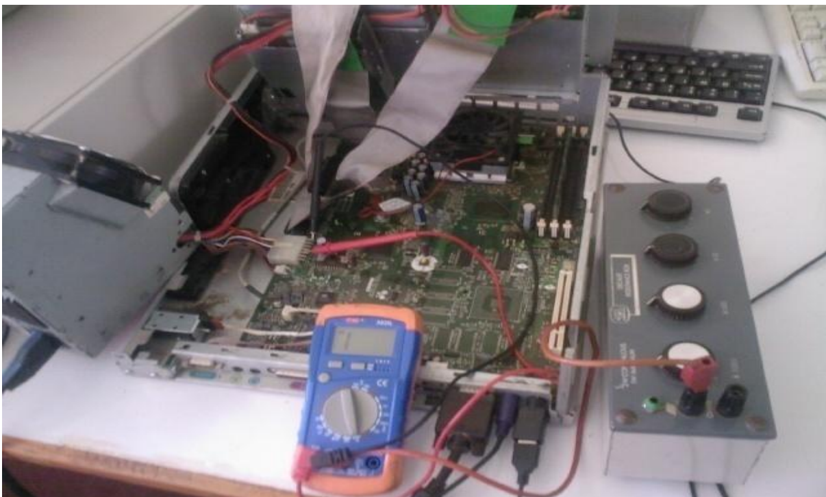
Plate A2: Voltage and Current measuring circuit for the Compaq desktop computers
