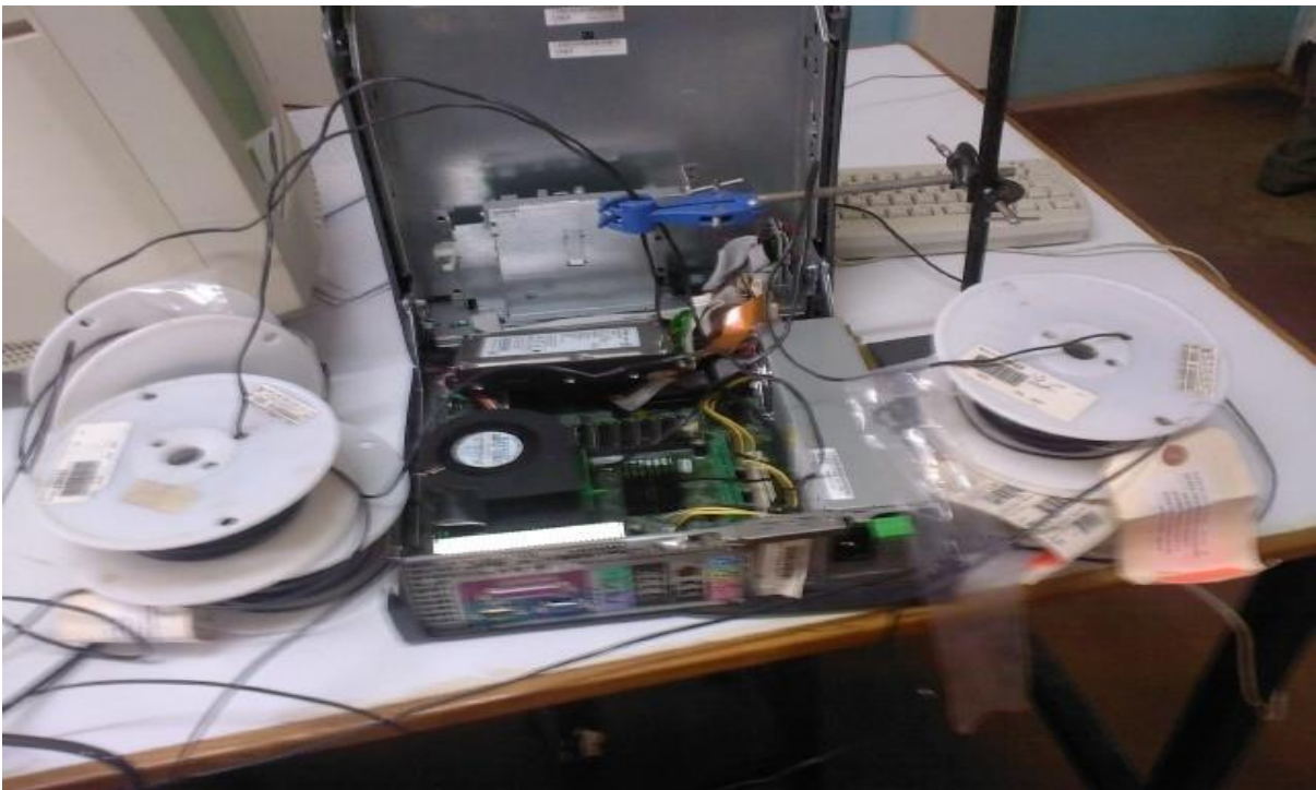
Plate B2; Thermocouples connected to the heat generation modules in the Dell desktop computer
