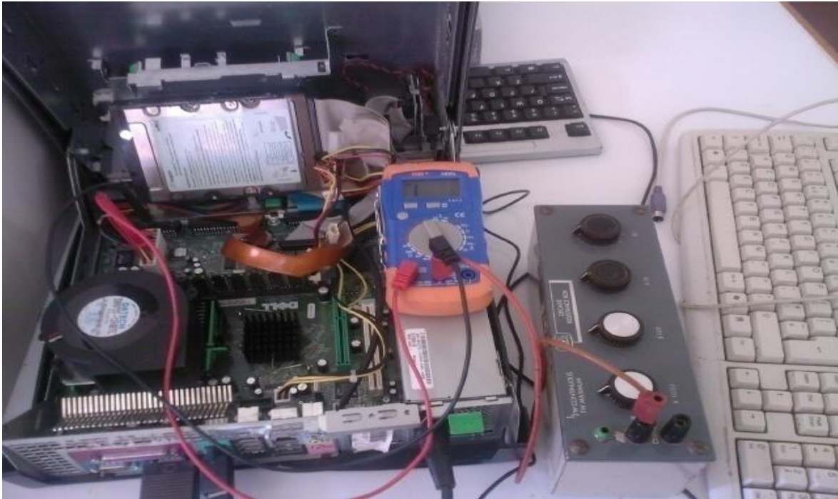
Plate A1: Voltage and Current measuring circuit for the Dell desktop computers
