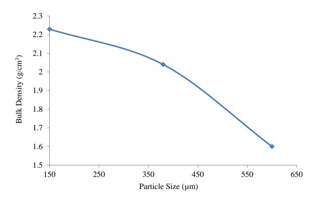
Figure 4.11: Effect of particle size on bulk density.
