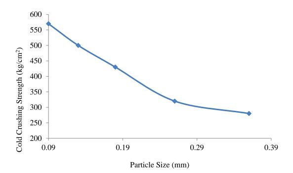
Figure 2.3: Effect of particle size on cold crushing strength. (Adopted from Aigbodion *et al.*, 2010).
