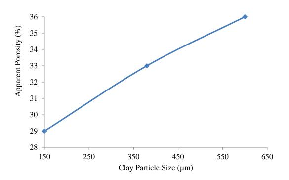
Figure 4.10: Effect of particle size on apparent porosity.
