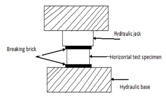
Figure 2.2: cross section of cold crusching
