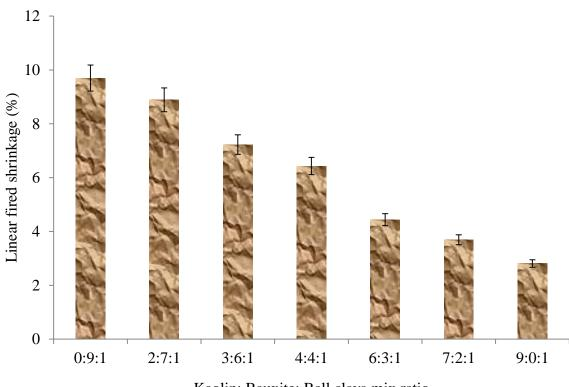
Kaolin: Bauxite: Ball clays mix ratio
