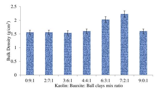
Figure 4.6: Effect of mix ratios on bulk density.
