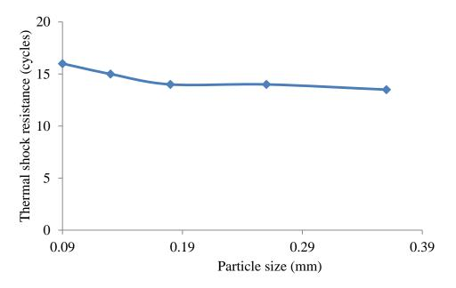
Figure 2.5: Effect of particle size on thermal shock resistance. (Adopted from Aigbodion *et al.*, 2010).
