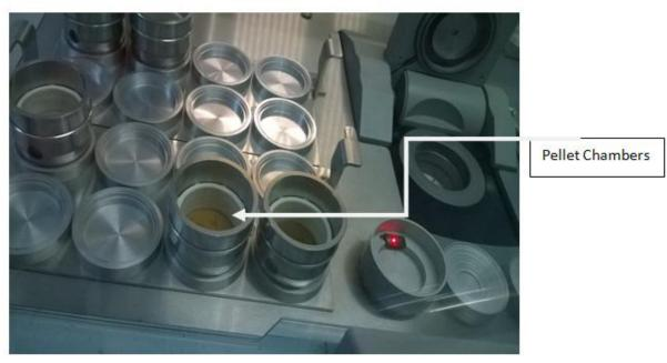
Plate A.4: X-ray pellet chambers
