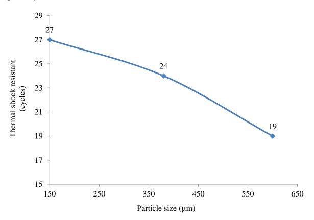
Figure 4.14: Effect of particle size on thermal shock resistance.
