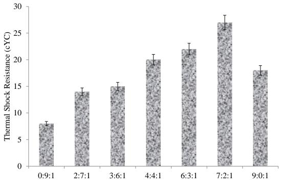
Kaolin: Bauxite: Ball clays mix ratio
