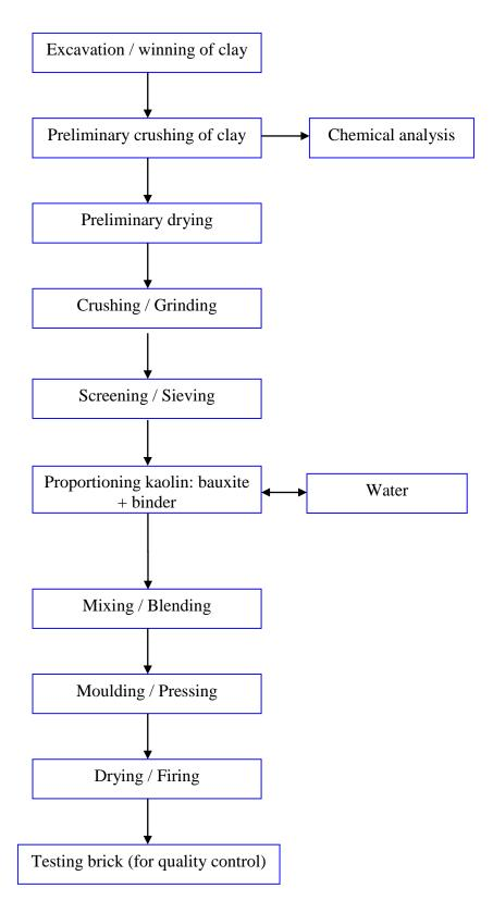
Figure 3.1: Production Flow chart and testing.
