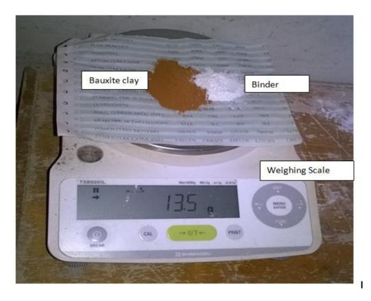
Plate A.2: Raw material clay (12g) and binder (1.5g)
