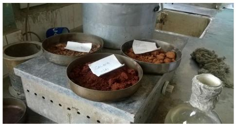
Plate A.1: Materials drying at 250°C
