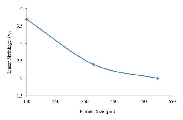
Figure 4.13: Effect of particle size on linear shrinkage.
