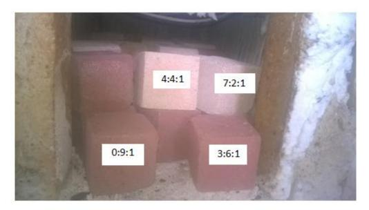
Figure 4.4: Fired bricks samples at different mix ratios.
