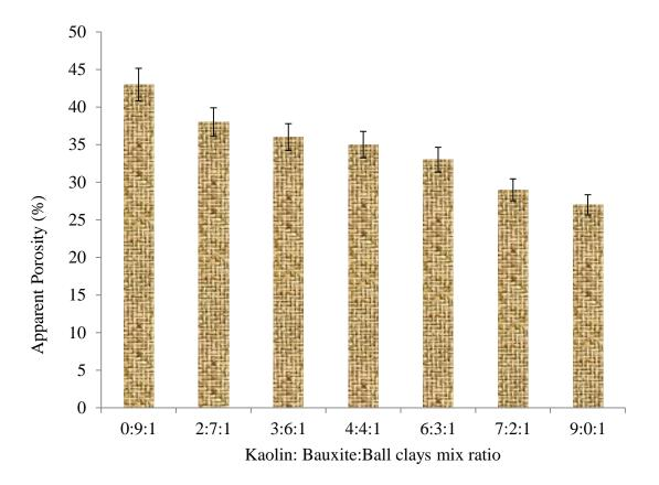
Figure 4.5: Effect of mix ratios on apparent porosity.
