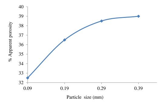
Figure 2.1: Variation of porosity with particle size. (Adopted from Aigbodion *et al.* 2010)
