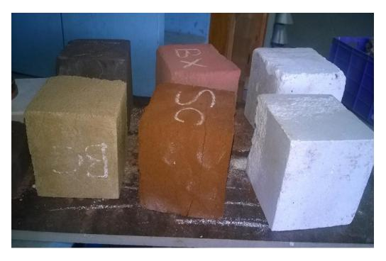
Figure 4.2: Fired bricks of individual clays.
