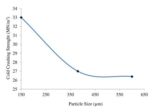
Figure 4.12: Effect of particle size on cold crushing strength.
