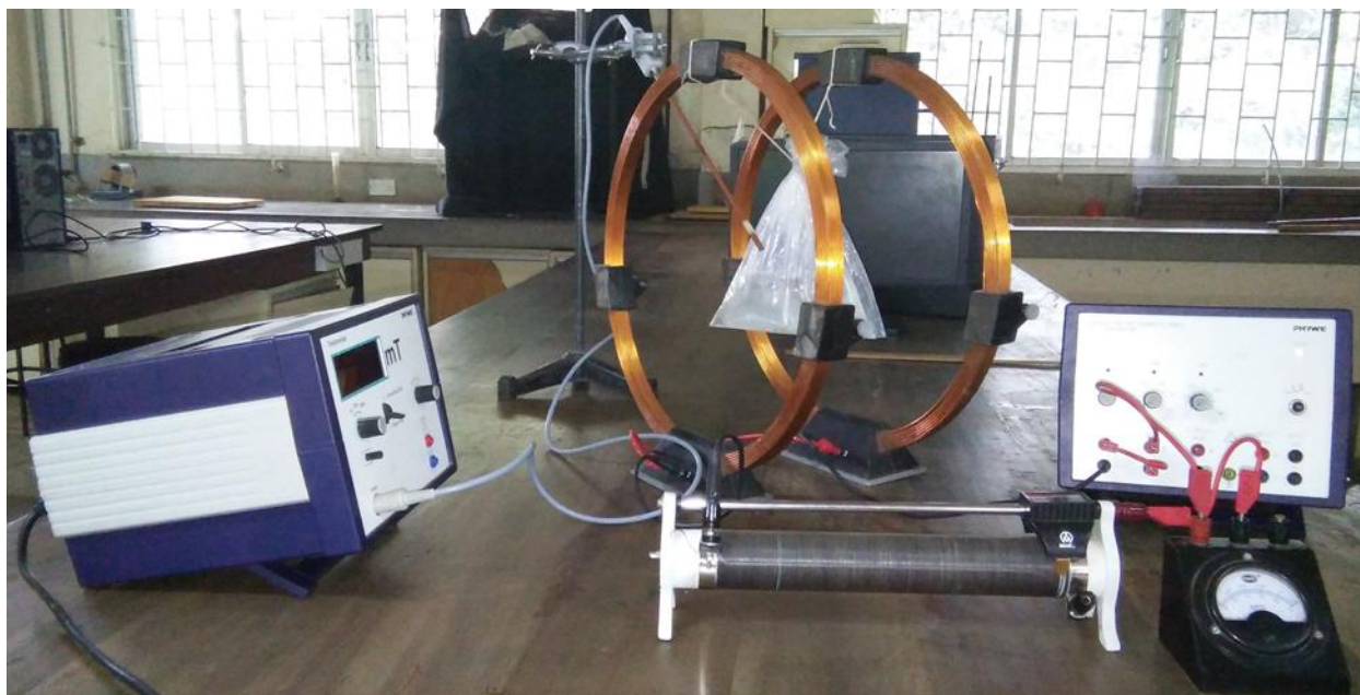
Plate 2: Experimental setup for water samples magnetic B-field application
