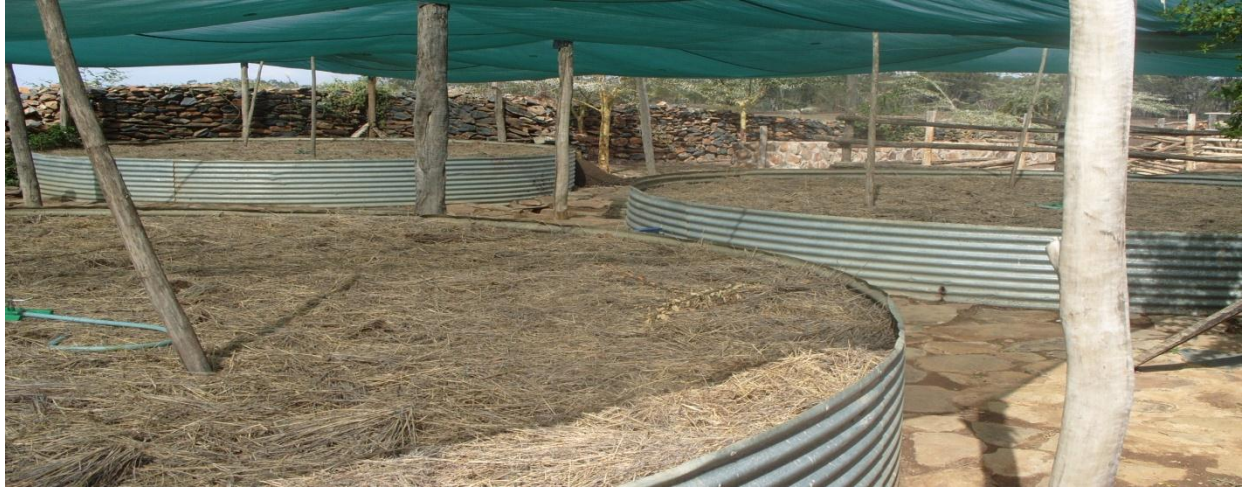
Plate 2: Photograph of biodegradation tanks for earthworm leachate production
