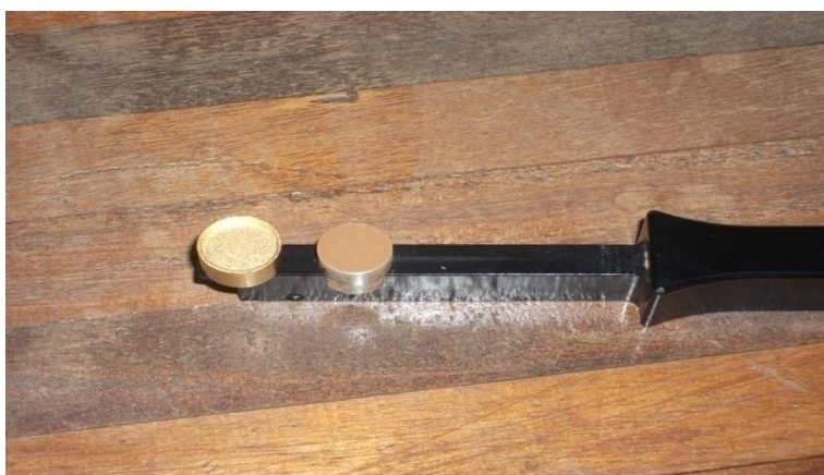
Plate 6: Photograph showing the sample rack, sample cup and the gold cup
