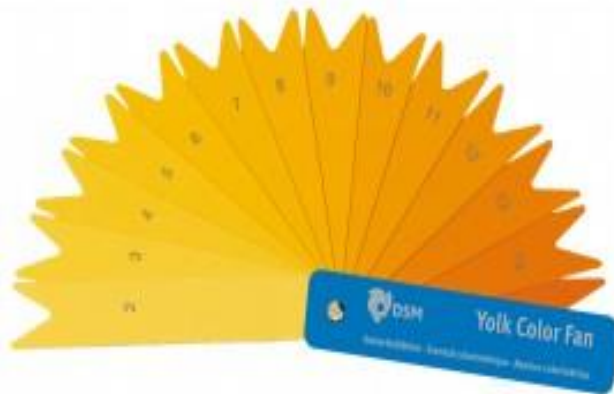
Fig 2- Yolk colour fan for yolk colour determination
