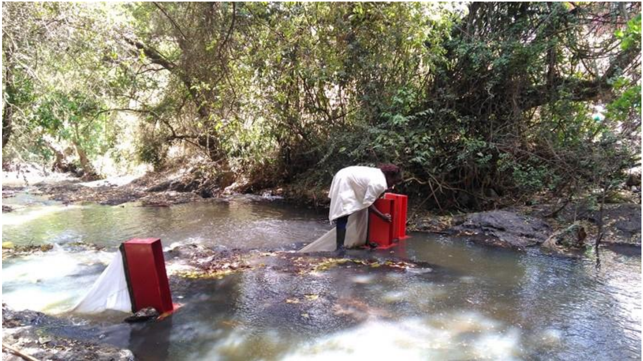
Plate 1: The riffle biotope in the Njoro River showing the drift nets facing upstream (Source: Photograph by the Author 23/01/2017).
