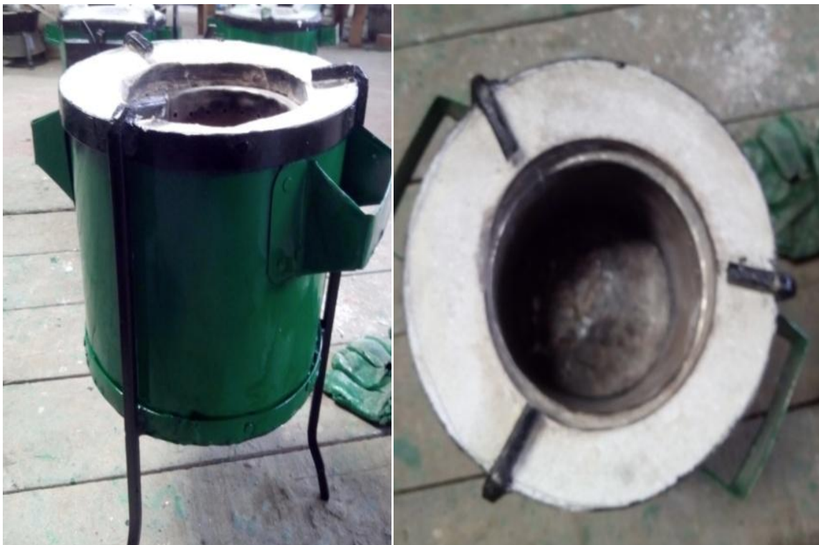
Figure 3B: Embodiment of the Developed Micro gasifier Stove
