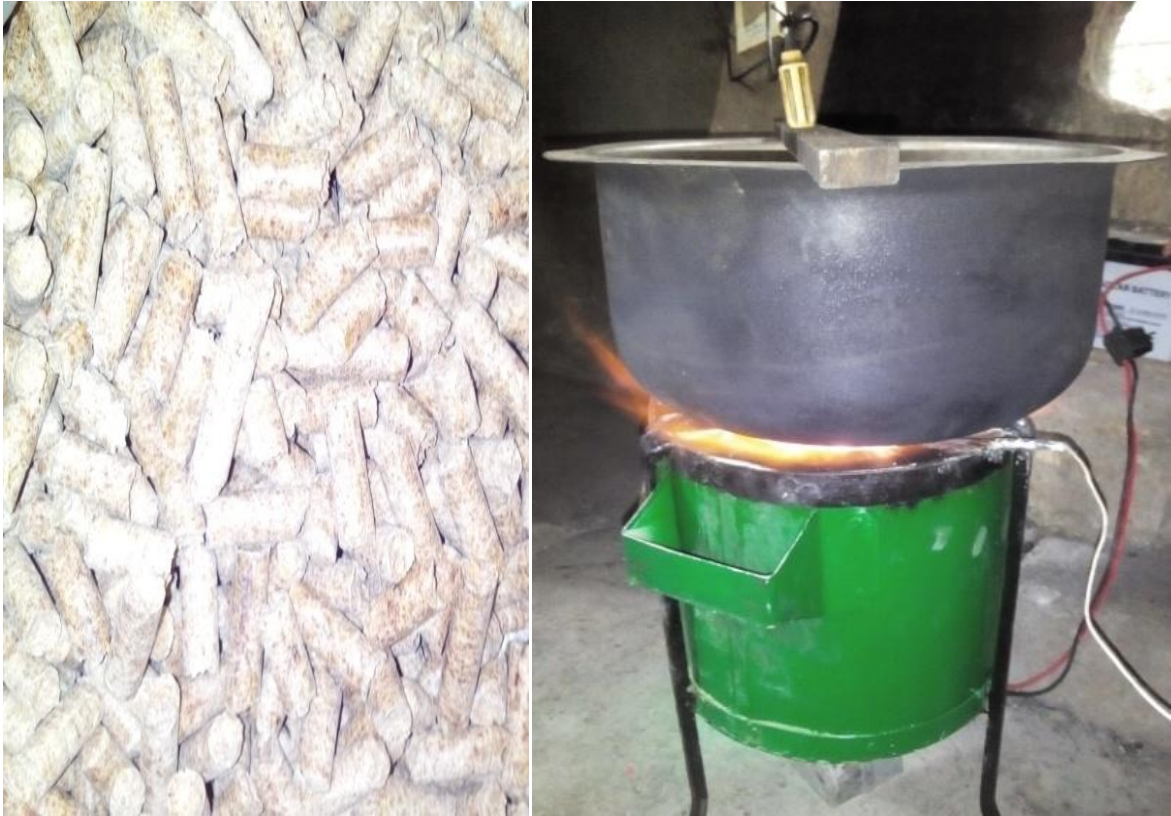
Figure 6A: Water Boiling Test Set Up and Saw Dust Pellets Used
